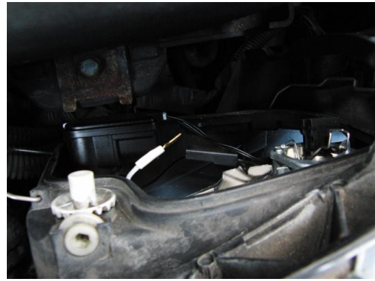
HIGH BEAM SUPPLY DISCONNECTED
