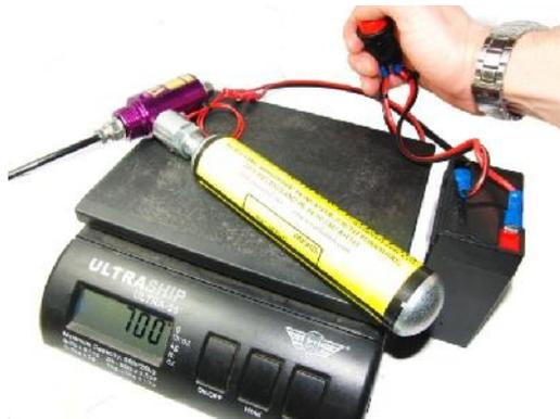
**ONLY A 'SWITCHED' SUPPLY MUST BE USED TO ENERGISE THE SOLENOID, DO NOT HOLD BARE WIRES TO A BATTERY AS IT WILL CAUSE SPARKS WHICH WILL IGNITE EVEN SMALL AMOUNTS OF LEAKED PROPANE.**
