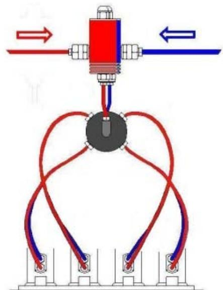
**WARNING; Never mount a D-Block any other way than described above, as it will result in uneven distribution leading to potential engine failure. If you feel it is impossible to mount the D-Block as described on your particular vehicle please contact us for assistance.**
